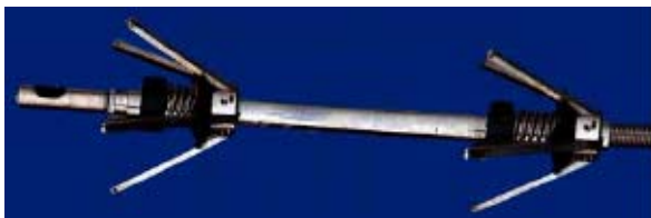
UT probe for tube inspection
